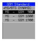
The default value DYNAMIC uses a fixed Power vs Time limit line template. Selecting GSM900, GSM1800 or GSM1900 (mobile station) the limit lines are calculated internally by taking into account special user settings as 'control level' and 'absolute level'.
